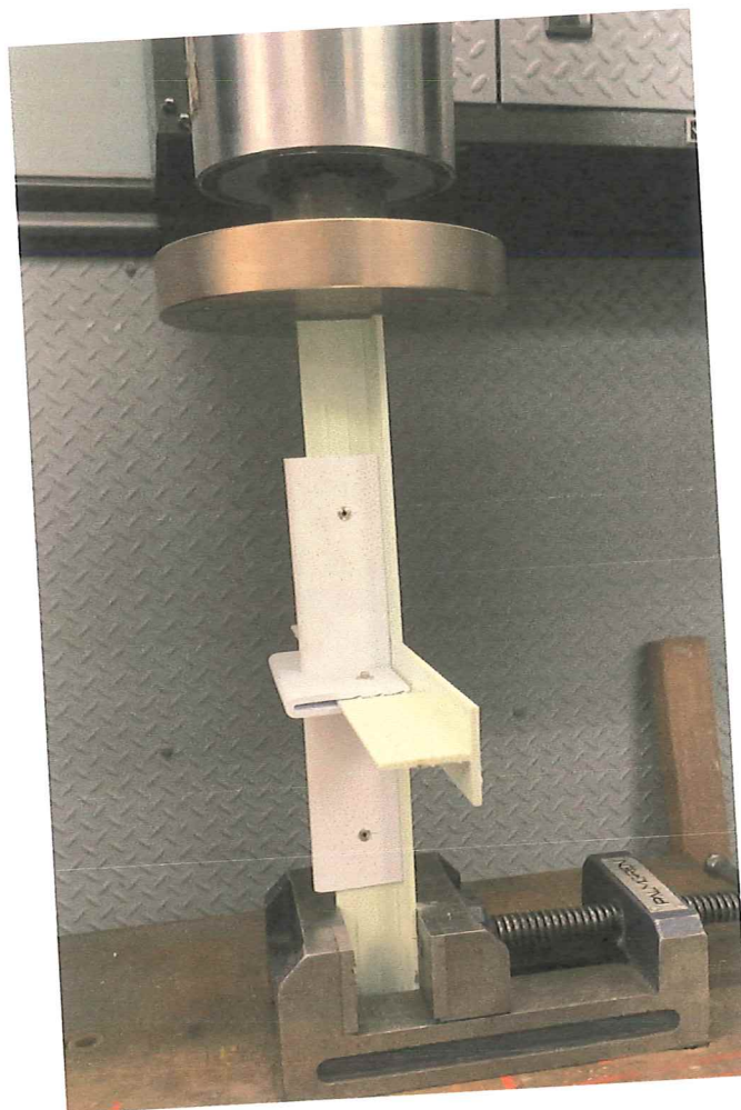
Cross Tee Clip System Compressive Test
