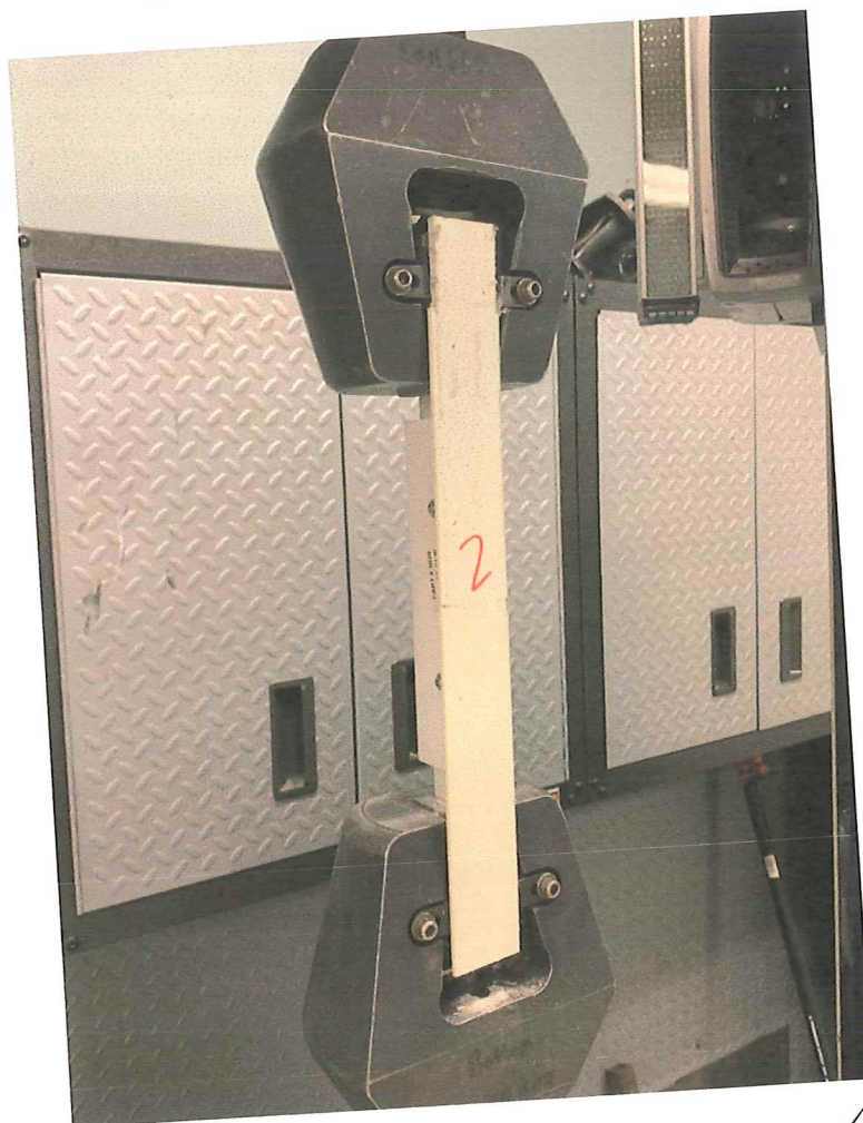
Splice Clip Pull-Apart Test
