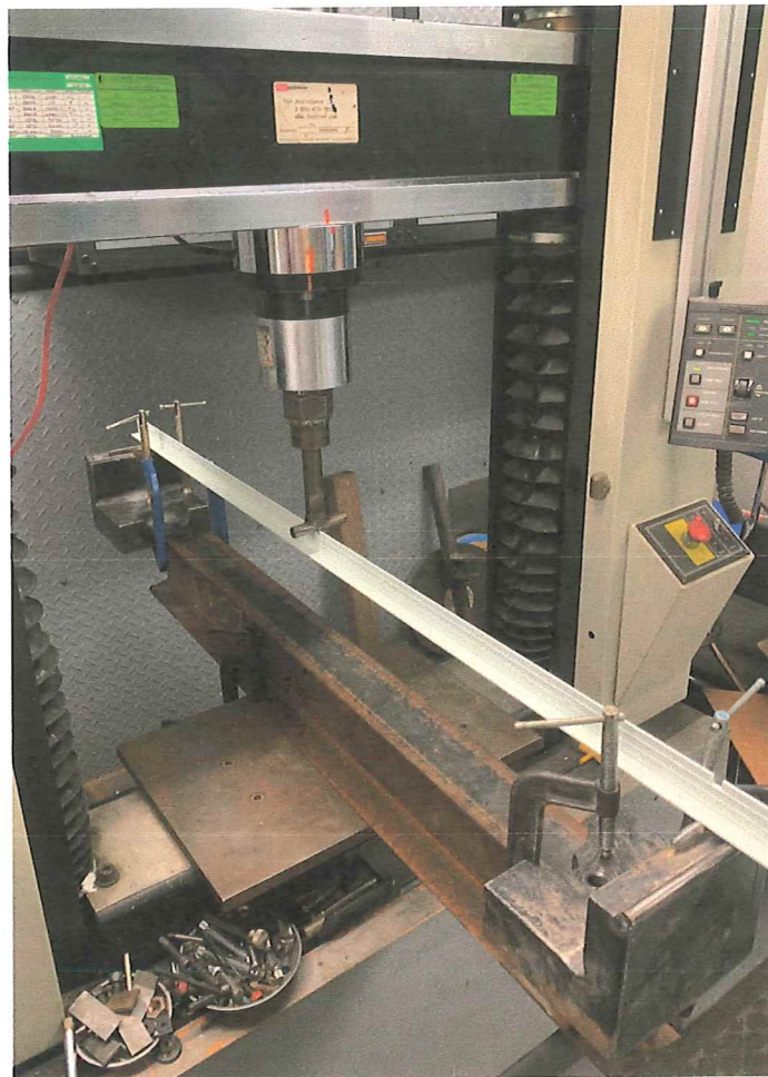
Tee Beam Strength Test
