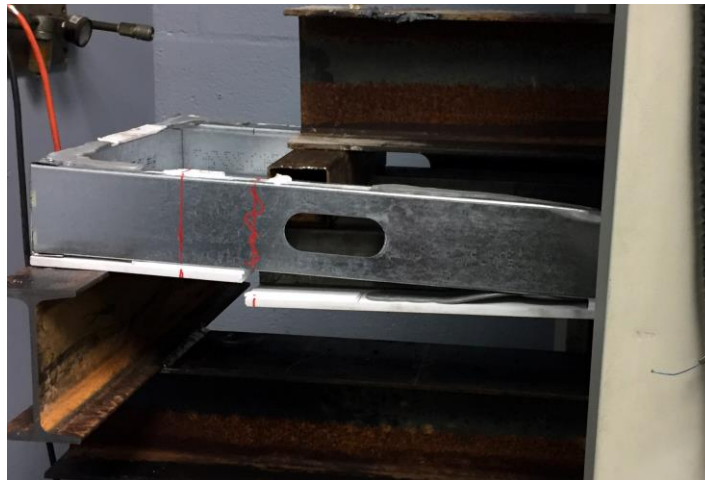
Figure 10: Sample #5,6 Typical Failure
